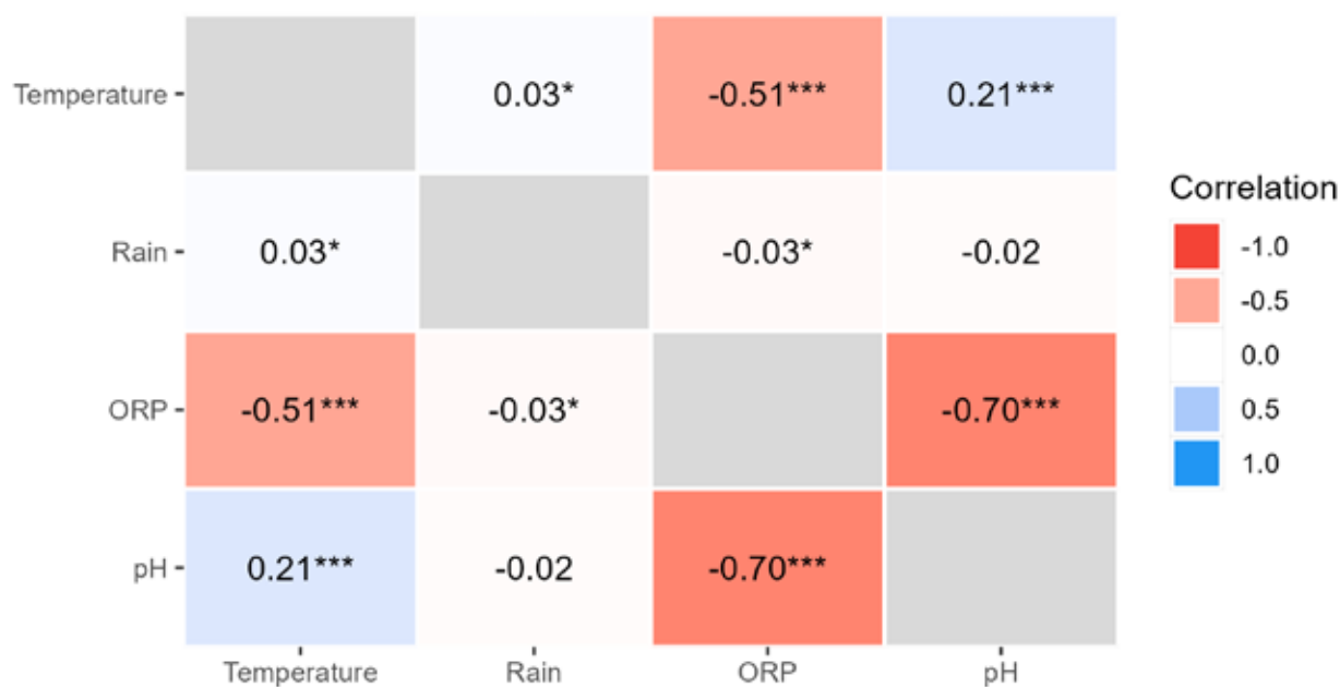
Figure 7: Spearman's rho correlation matrix demonstrating the degree of association between ambient air temperature, rainfall, ORP, and pH.
